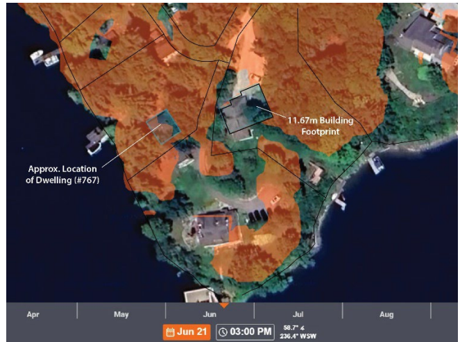
Figure 6c – Shadowing Impacts from an 11.67m Structure at 761 Christie Lake Lane 32D (3pm - June 21 st )
